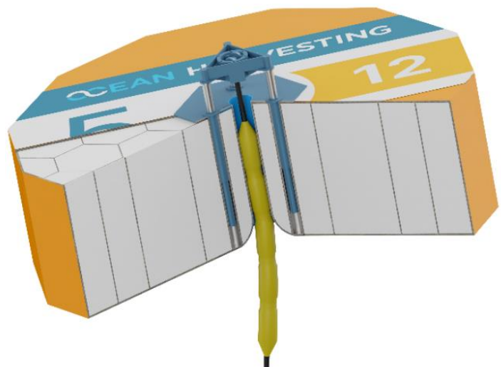
OHT's buoy with thin-walled honeycomb structure of high-performance concrete and EPS cores.
